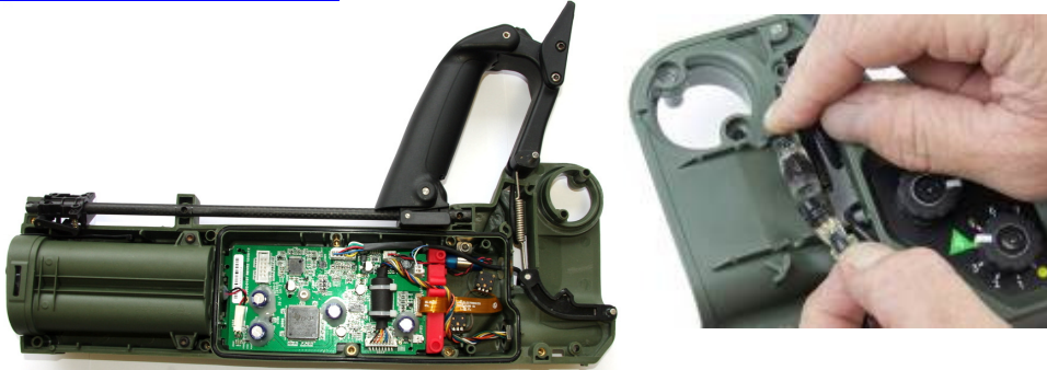
Figure 78: Disconnect Wiring Loom Handle
