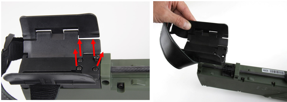
Figure 8: Removing the Armrest
