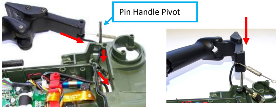
Figure 81: Threading the Wiring Loom
