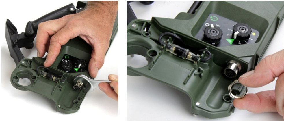
Figure 31: Removing the Coil Connector Nut (18mm)
